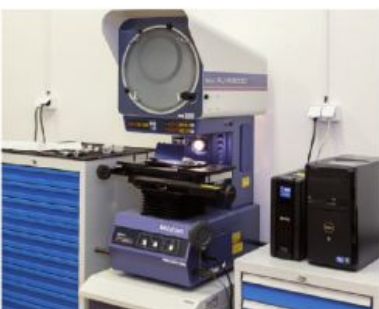
Profile projector at the Quality Management Laboratory.
