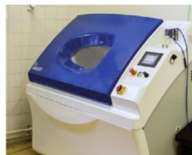
Corrosion chamber to simulate extreme conditions for material testing.
