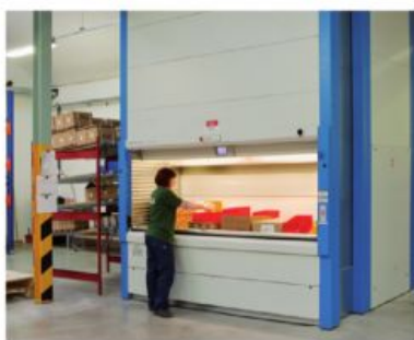
Kardex: automated high-capacity storage system.
